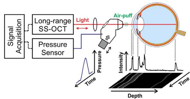
**FIGURE 1.** Scheme of the prototype SS-OCT ocular biometer. The system can acquire simultaneously the OCT A-scans in time (M-scan) and corresponding air-puff pressure acting on the cornea. The pressure is later converted into the force based on the sensor calibration.
